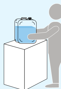
Lifting block: allows lifting the container from floor to head in two actions and allows people to sit and rest
